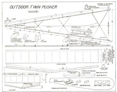
The new built-up frame gives additional strength without increasing weight.
